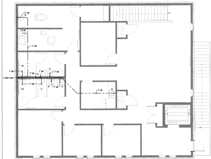
2ND FLOOR PLUMBING WASTE PLAN - SCALE: 1/4" = 1' 2
