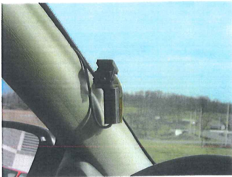
Figure 9. Driver Face Camera, Mounted near the left A-Pillar.
