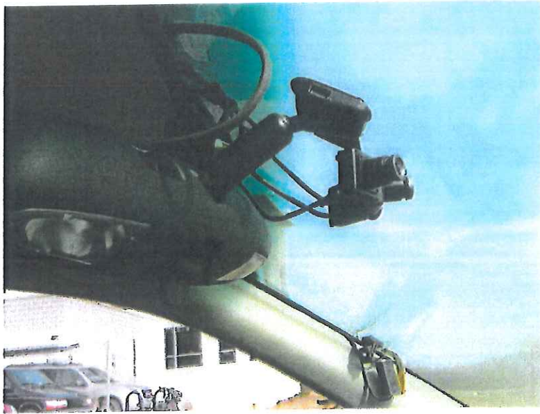
Figure 8. Forward Facing Cameras Mounted Behind the Center Rear View Mirror.
