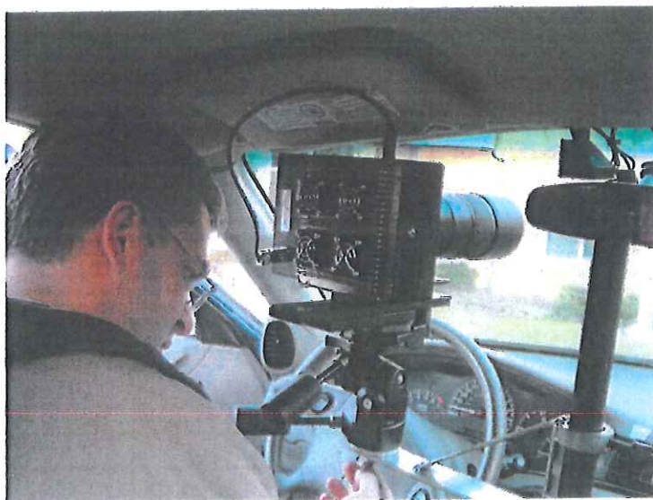
Figure 35. Radiant Imaging CCD Photometer in Position for Measurements, with Experimenter Making Final Adjustments.
