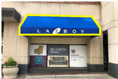
Awning sign area is computed based on total height and width of viewable portions of the awning face
