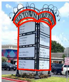
Multi-Faced Signs – Sign area computed on sign faces visible from any one point
