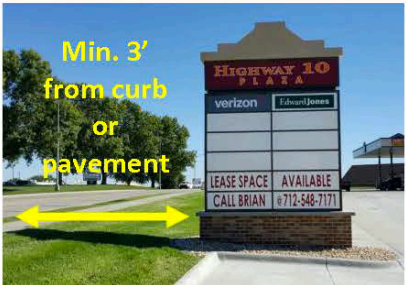
No part of sign may be closer than 3 feet to a curb or street pavement measured horizontally from curb to sign
