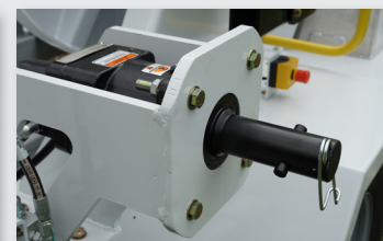
Spider® Pilot Line System with independent levelwind
