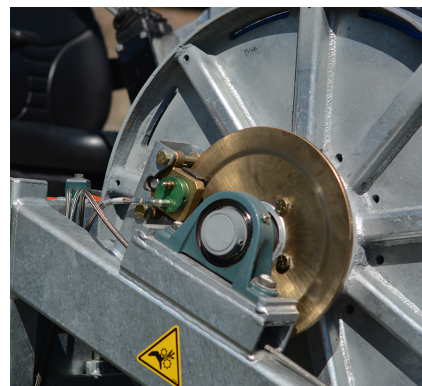
Braking system with electric over hydraulic activation
