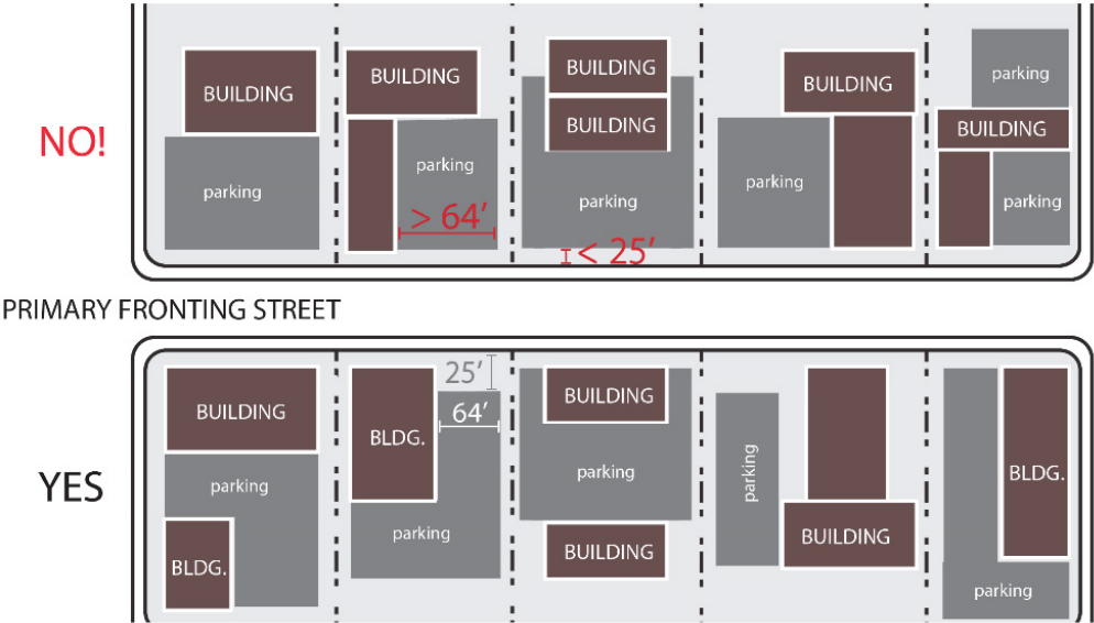
FIGURE 3.5.9.D1, PARKING LOT CONFIGURATION
